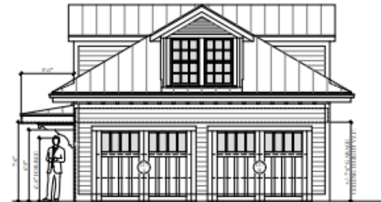
06 PROPOSED SOUTH ELEVATION 1/4" = 1'-0"
