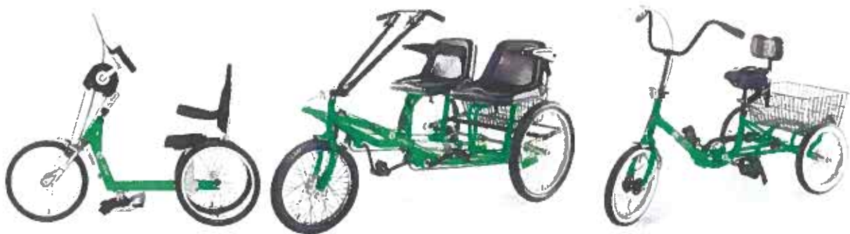
(L-R) Seated Handcycle, Dual seated pedal powered three-wheeler, Compact balance stability tricycle
