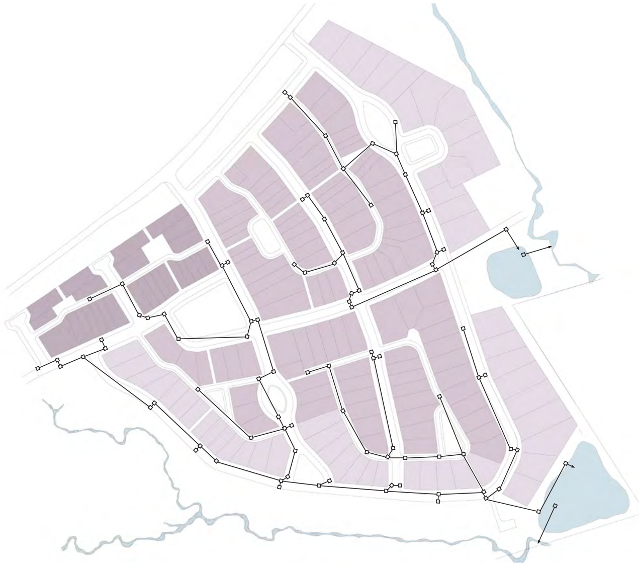
CONVENTIONAL TND STORM WATER PLAN
