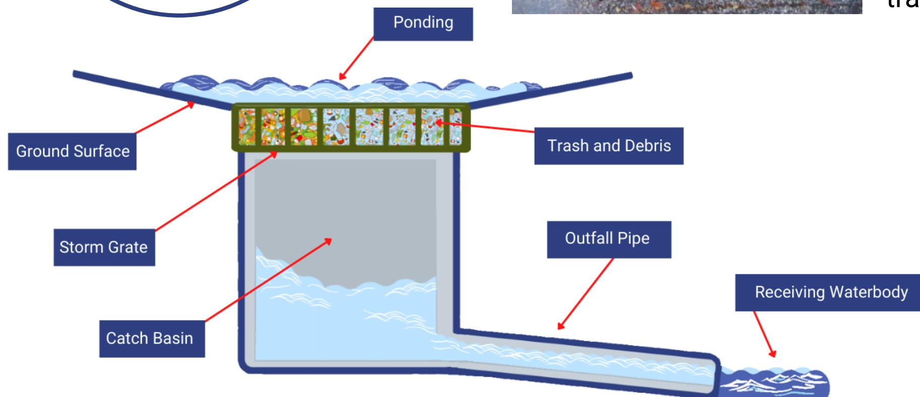
Trash and debris caught on and in the storm grate causes ponding on the surface.
